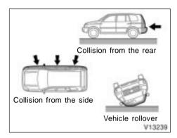
The SRS front airbags are generally not designed to inflate if the vehicle is involved in a side or rear collision, if it rolls over, or if it is involved in a lowspeed frontal collision. But, whenever a collision of any type causes sufficient forward deceleration of the vehicle, deployment of the SRS front airbags may occur.
