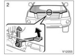
2. In front of the vehicle, pull up the auxiliary catch lever and lift the hood.
