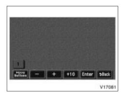
Enter the disc menu number by using the "-", "+" and "+10" switches and push the "Enter" switch. The player starts playing the disc from the entered disc menu number. The entered disc menu number will appear on the screen.
