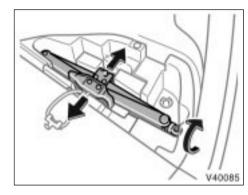
To store the jack, rotate the jack joint until the jack is firmly secured.
