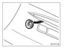
EJECTING THE DISC Push the "**≜**" button.
