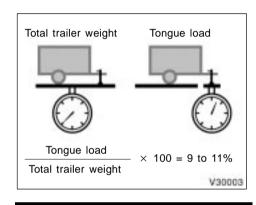
The trailer cargo load should be distributed so that the tongue load is 9 to 11% of the total trailer weight, not exceed the following.
