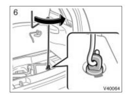
6. Threading the jack handle through the adapter socket, turn the jack handle counterclockwise. Continue until the spare tire is lowered completely to the ground.
