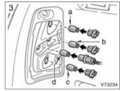
a: Stop/tail light b: Rear turn signal light c: Stop/tail light d: Back- up light
