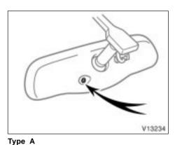
To ensure correct functioning of an anti-glare mirror sensor located on the back side of the mirror, do not touch or cover the sensor with your finger or a piece of cloth, etc.
