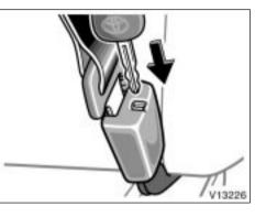
To release the concave end tab, insert the key into the hole on buckle 1 and allow the belt to retract.
