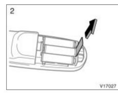
2. Remove the insulating sheet.
