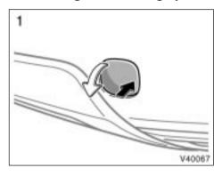
1. Remove the front towing eyelet cover on the front bumper by pushing the outside of the cover.
