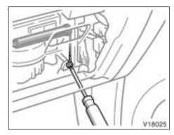
1. Remove the clip with a Phillips-head screwdriver.
