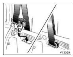
To stow the third seat seat belt, insert the tabs into the slot as shown above. Make sure the tabs are securely locked in the slot.
