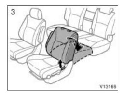
3. Pull the seatback angle adjusting lever up to unlock and push down the seatback.
