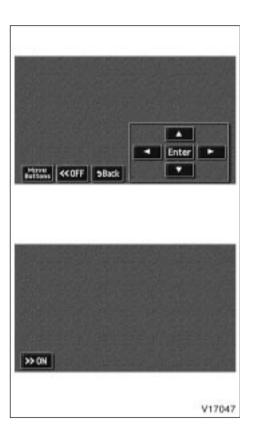
To select the menu for the disc, push the " $\blacktriangleleft$ ", " $\bigstar$ ", " $\bigstar$ " or " $\blacktriangledown$ " switches on the screen. Push the "Enter" switch to select the menu for the disc.
