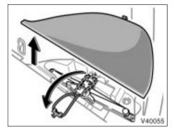
Before removing the jack, remove the right side deck board and unhook the tightening strap.
