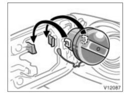
3. The removed cap can be stored on the back side of the fuel filler door.
