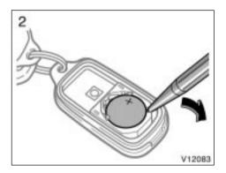
2. Remove the discharged transmitter battery by ballpoint pen. Insert the tip of ballpoint pen at the guide groove and lift as shown in the above illustration.
