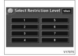
Push a parental level (1—8). The smaller the level number, the stricter the age limit. Push the "Back" switch to return to the "Setup Menu 1" screen.
