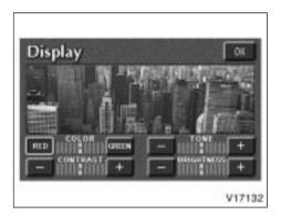
Each time you push the "+" or "-" switch, you can adjust the color, contrast, tone and brightness of the screen.
