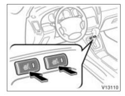
To turn on the seat heater, push the switches ("L" switch for the left front seat and "R" switch for the right front seat). At this time, the indicator light will illuminate to indicate the seat heater is operating.
