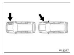
The SRS side airbag and curtain shield airbag system may not activate if the vehicle is subjected to a collision from the side at certain angles, or a collision to the side of the vehicle body other than the passenger compartment as shown in the illustration.
