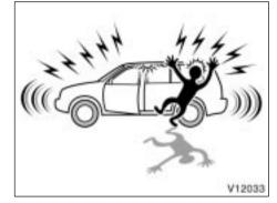
To deter vehicle theft, the system is designed to sound an alarm if any of the side doors, back door or hood is forcibly unlocked or the battery terminal is disconnected and then reconnected when the system is set.
