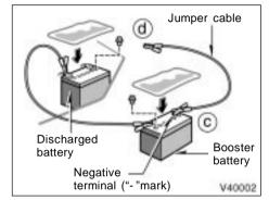
c. Connect the clamp of the negative (black) jumper cable to the negative (-) terminal on the booster battery.
