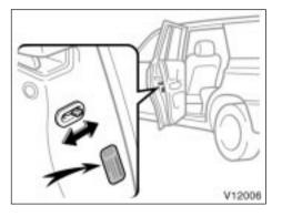
REAR DOOR CHILD-PROTECTORS Move the lock lever to the "LOCK" position as shown on the label.
