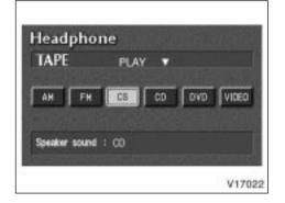
The mode display which is selected by the joystick is colored blue. When the "ENT" button is pushed, the mode display changes to green. If the mode display is gray, it cannot be selected.
