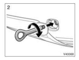
Use the front towing eyelet in the luggage compartment. Secure it to the hole on the bumper by turning clockwise. (For the towing eyelet location, see "—Required tools and spare tire" on page 330 in this Section.)
