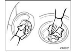
Before putting on wheels, remove any corrosion on the mounting surfaces with a wire brush or such. Installation of wheels without good metal- to- metal contact at the mounting surface can cause wheel nuts to loosen and eventually cause a wheel to come off while driving.
