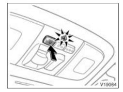
The garage door opener (**HomeLink**<sup>®</sup> Universal Transceiver) is manufactured under license from HomeLink<sup>®</sup> and can be programmed to operate garage doors, gates, entry doors, door locks, home lighting systems, and security systems, etc.
