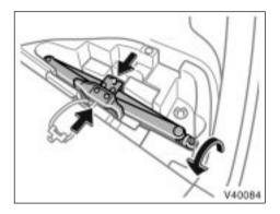
To remove the jack, rotate the jack joint by hand until the jack becomes free.
