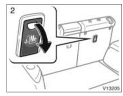
2. Open the anchor bracket cover with the symbol as shown in the illustration.
