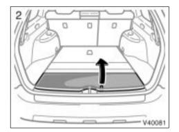
2. Pull the strap and open the center deck board.
