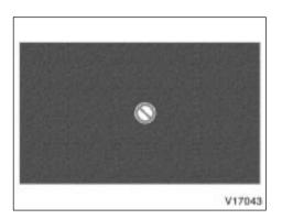
If "0" appears on the screen when you select a switch, it indicates that the switch cannot work.
