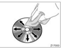
To clean a compact disc: Wipe it with a soft, lint-free cloth that has been dampened with water. Wipe in a straight line from the center to the edge of the disc (not in circles). Dry it with another soft, lint-free cloth. Do not use a conventional record cleaner or anti-static device.
