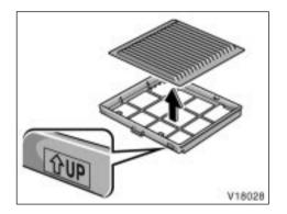
5. Remove the filter from the filter case.
