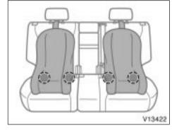
Lower anchorages for the child restraint systems complying with the FMVSS225 or CMVSS210.2 specifications are installed in the second seat.
