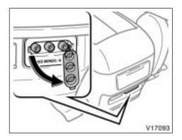
To use the input terminal adapter, open the cover.
