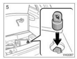
5. Put the adapter socket (for removing a spare tire) on the spare tire clamp bolt.
