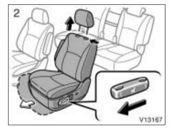
2. Remove the head restraint. Push the seat position adjusting switch forward to slide the front seat to the front-most position.
