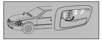
c. The tail and marker lights flash 1 time, the buzzer chirps 1 time, and the doors lock and unlock 1 time. →
