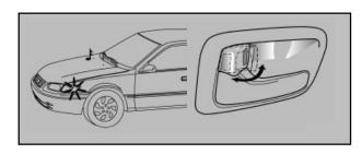
The tail and marker lights flash 1 time, the buzzer chirps 1 time, and the doors lock and unlock 1 time.\*
